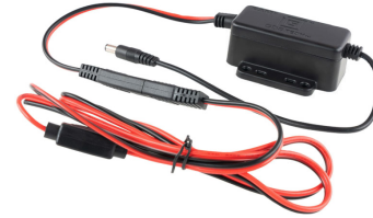
RAM-GDS-CHARGE-V9U GDS® 20-60VDC Input (12VDC Output) Hardwire Charger with Male DC 5.5mm
