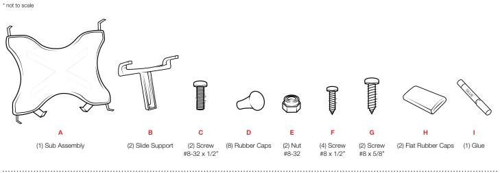
Attach (D) and (H) Rubber Caps to each prong on (A) Sub Assembly. Use optional (I) Glue for a secure hold.
