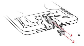
Using floss, fishing line (recommended) or a credit card, insert between **(A) Tab-Conn**<sup>™</sup> and tablet to gradually separate each adhesive from back of tablet. Use cleaner for any remaining adhesive residue.
