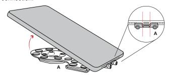
Connect straight end of (C) USB-C Cable into back of (A) **Tab-Conn**<sup>™</sup>. Connect 90-degree angle side of cable into the USB port of your tablet.
