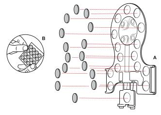
Carefully peel away remaining film from each (B) Adhesive Pad.
