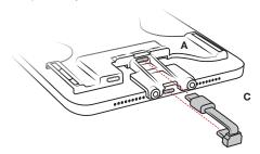
Insert (D) Cable Cover into back of (A) Tab-Conn™, clicking into place and covering USB connection.
