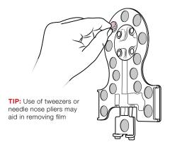
While holding upside down, align bottom of (A) Tab-Conn™ to be centered with the USB-C port of your tablet. Keep angled away to prevent adhesives from making contact with tablet. Once fully aligned, bring (A) Tab-Conn™ in to adhere to back of tablet. Press firmly and evenly for proper connection.
