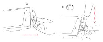
With nuts facing up, insert bottom connector into (A) Thin-Case™ Body, simultaneously plugging the connector into the tablet. Click components together to secure. Install (B) Machine Screws into the back holes of (A) Thin-Case™ Body. Fully tighten.
