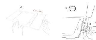
With nuts facing up, insert (B) Plug Insert into (A) Thin-Case<sup>™</sup> Body, simultaneously plugging the connector into the tablet. Click components together to secure. Install (C) Machine Screws into the back holes of (A) Thin-Case<sup>™</sup> Body. Fully tighten.
