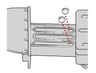
Attach (M) screws from behind the internal slide. Do not fully tighten (slides must remain loose)
