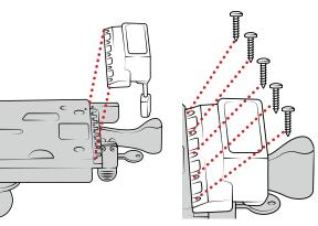
Using (K) screws, attach top docking cup to top slide with numbers facing down.
