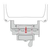
Press down on top cup to secure over tablet.
