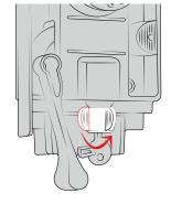
Insert top slide over internal vehicle dock.
