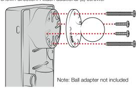
Using (K) screws, attach bottom docking cup to vehicle dock assembly.
