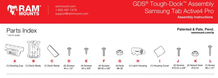
Connect (A) Docking Cup to (B) Dock Body using (D) Screws. Then Connect Dock Ramp to (B) Dock Body using (E) Screws.
