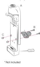
Insert your phone with IntelliSkin® into (A) Dock with top cup seated comfortably over your phone. Key lock must be in locked position.
