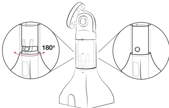
4 With **(D) Base Cover** and **(E) Tube Cover** positioned over **(C) Base Plate**, press **(B) Top Post** into hole, aligning the press-button with the desired hole determined in Step 3.
