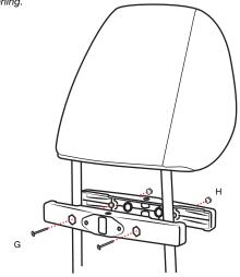
Connect (B) Swivel Hinge to center hole of (A) Clamp Base Half using (I) Bolt, (H) Washer and (G) Knob, as shown. Configure the angle and direction to best conform to car seat.
