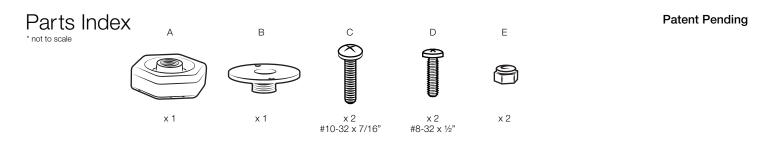
Connect Diamond Ball Adapter to the two-hole pattern of the (A) RAM® Vibe-Safe<sup>™</sup> using (C) Screws.
