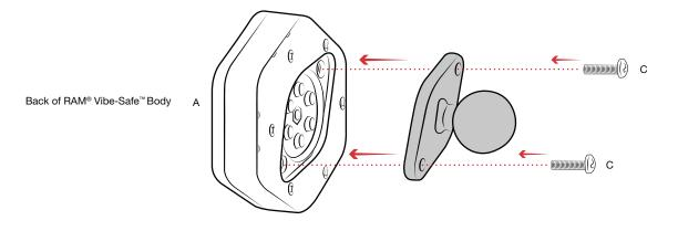
Connect RAM® X-Grip® to front side of (A) RAM® Vibe-Safe™ using (B) Screw. Optional tether is recommended for any rough environments and/or open cockpit applications. To apply tether, wrap around back of RAM® X-Grip® housing before connecting to RAM® Vibe-Safe™.
