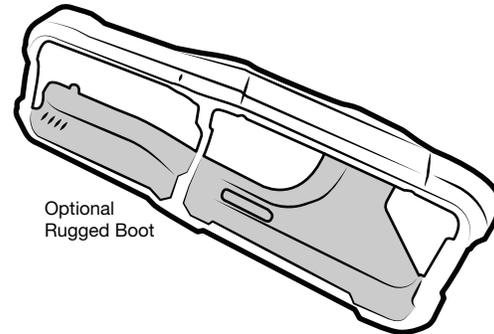
1 If your Zebra MC9300 does not have a Protective Boot, insert (B) and (C) Inserts into the top and bottom cups of (A) Holder. If your device has the Protective Boot installed, do not use inserts.
