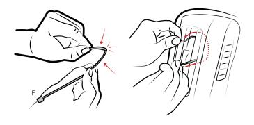
Apply (A) Vent Connector, routing (F) Zip Ties evenly through the center. Tighten zip ties to secure in place and trim excess.
