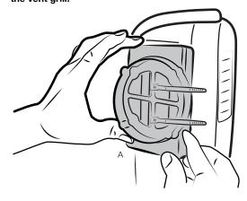
Connect (C) 90-Degree Hose Adapter to the back of your 4 dock, and (E) Grill to the front of your dock, using the (G) Screws and (H) Nuts
