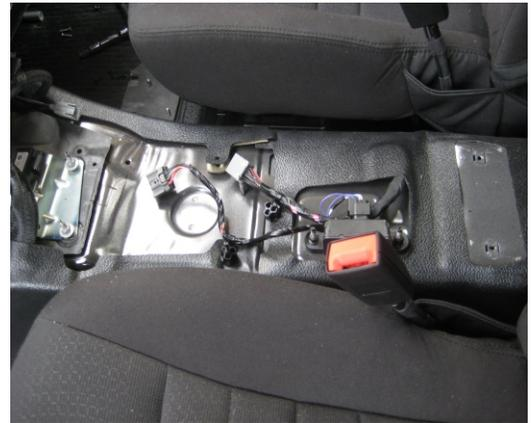
The area between the front seats must be accessible in order to install the console and fairing.
