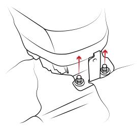
4 Using a 1/2" socket, loosen the two nuts on the studs at the rear of the seat tower bracket. The nuts need only be loosened so that they are approximately 1/2" above the surface.
