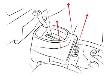
3 Locate the final retaining clip or Phillips screw and remove. Once out, the shift tower cover can be removed easily. Lift out the shift tower and store it along with the cup holder and all related hardware. Keep safe for re-installation.
