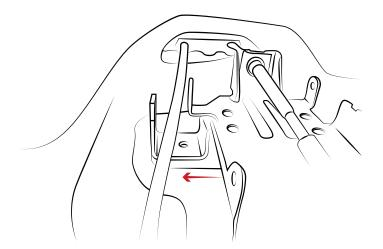
7 Position the No-Drill base so that the holes are aligned and reposition both the bracket and base over the mounting holes in the floor pan.
