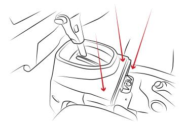
10 Lower the shift tower cover back over the shift tower. Re-place the retaining clips previously removed and re-install the cup holder.
