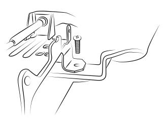
3 With the mounting holes aligned, re-insert the mounting bolts and begin thread by hand.
