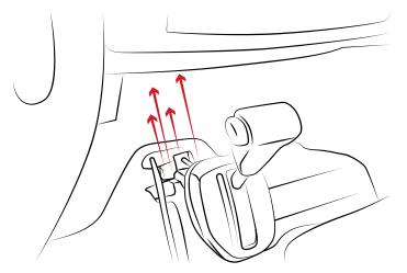
5 Locate the brackets and mounting bolts at the front of the shift tower. The 4 bolts located there will need to be removed for installation.
