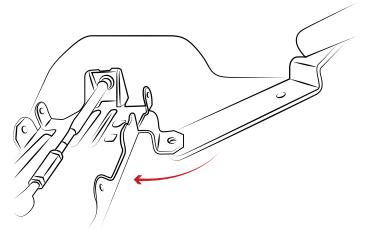
6 With the mounting bolts holding the shift tower brackets removed, lift the brackets so that a 1/4" gap is created between the floor pan and the shift tower bracket. Slide the No-Drill base between the shift tower bracket and the floor pan.
