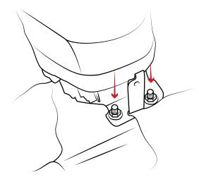
9 With all of the mounting bolts started by hand, use a socket wrench or powered drill type tool to fully tighten the bolts and nuts previously loosened.
