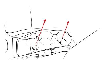
2 In some model years, there will be a Phillips screw or retaining clip located under the front of the cup holder. Remove these screws, pull the E-Brake and lift out the cup holder.
