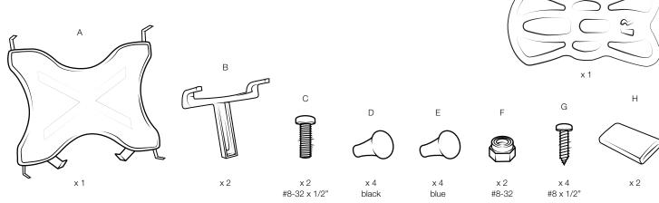
1 Attach (E) blue rubber caps to each prong on (A) sub assembly.
