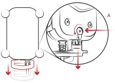
Insert and secure (B) Leg Cover when not using the support leg
