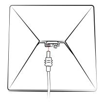
Insert the Ball Adapter into the Starlink Mini until it 'clicks' into place.
