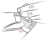
Repeat on opposite tab of the Ball Adapter. While sliding outward, the Ball Adapter should become disconnected completely from the Starlink Mini.
