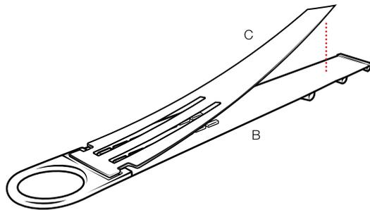
2 Cut out measuring strip shown on the right. Wrap the strip around area where RAM® EZ-Strap™ is to be attached until the "ALIGN EDGE WITH ZONE" end aligns with one of the "Short, Medium, or Long" segments to determine appropriate strap length. Once correct segment is determined, use scissors to cut only along one of the shown reference lines "....." just past the corresponding groove.
