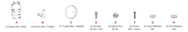
Insert phone into (A) Quick-Grip™ Body. Determine best placement of (B) Fingers to avoid blocking buttons.
