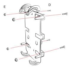
3 Attach Quick-Grip™ to (C) Tough-Mag™ Adapter using (F) Screws, (G) Washers, and (H) Washers.
