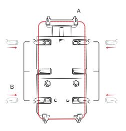
Remove phone and attach (B) Fingers using (D) screws and (E) nuts. Insert phone again, position the fingers flush against device and fully tighten screws from behind.
