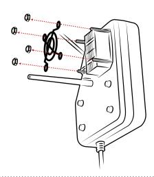
Reassemble (A) RAM® Temp-Right $^{\text{\tiny M}}$  to dock as shown. Dock style may vary
