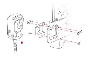
Connect (D) Double Ball Mount to (E) Backing Plate using (F) Backing Plate Hardware Pack.
