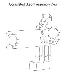
Connect (C) Double Ball Mount to (E) Backing Plate using (F) Backing Plate Hardware Pack.
