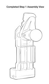
2 Connect (D) Double Ball Mount to (E) Backing Plate using (F) Backing Plate Hardware Pack.
