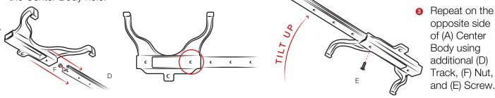
Onnect (B) and (C) ends to the opposite ends of (D) Tracks using the remaining (E) Screws and (F) Nuts. Hooks on (A), (B), and (C) parts should face the same direction.
