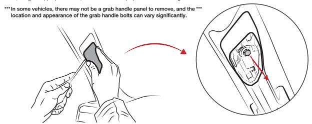
With the original grab handle bolt removed, attach the (A) RAM® Ball with (B or C) Bolt and (D) Lock Washer.
