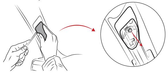
With the original grab handle bolt removed, attach the (A) RAM® Ball with (B) Bolt and (C) Lock Washer.
