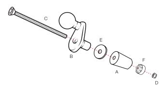
Insert assembly into fork stem hole until ball plate is flush with your bike. Tighten (C) Screw using a 3mm allen wrench. Periodically check the friction of the assembly to ensure it is tightening properly. If your assembly is not tightening, the (F) Nut Pocket Washer may not be gripping on the expansion plug. Remove assembly from hole and pre-tighten further, then repeat.
