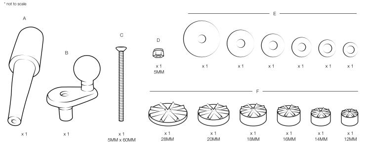
Measure inside diameter of fork stem to determine which side of the (A) expansion plug your install requires.
