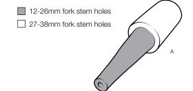
Gently insert the side of the (A) expansion plug that was determined in Step 1 into the stem hole and mark approximately 1/8" above the opening. Remove plug and cut marked line. Measure 1" below the top cut and cut along that line as well. Fork stems with a diameter of 20mm-26mm and 32mm-38mm will not require the 1/8" offset and will utilize the largest 1" section of the corresponding section of plug.
