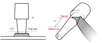
O Assemble components as shown before using appropriate (E) Washer and (F) Nut Pocket Washer. Diameter of selected (E) Washer must not be wider than diameter of the top cut of (A) Expansion Plug. Tighten assembly until (F) Nut Pocket Washer has a firm grip on (A) Expansion Plug.
