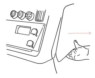
Connect ball base to any 4-Hole AMPS pattern using (E) Screws and (F) Washers.
