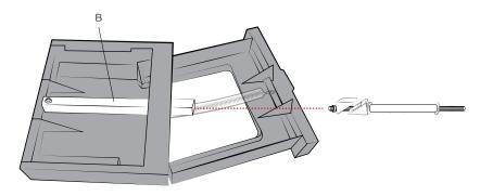
Olose Main Tray Slide slowly while feeding the end of Rod Assembly through (E) flange. Place (M) washer on the end and attach (P) RAM® Pin-Lock Nob all the way. Secure the Rod Assembly with (O) washer and (K) screw through the smaller hole on the (B) tube.
