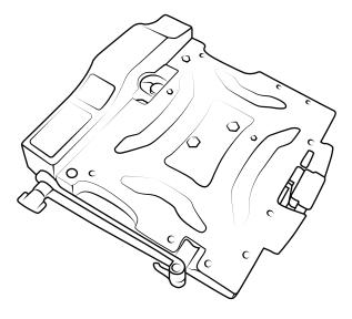
2 Pull latch forward until lock engages. Turn lock clockwise to lock and counter-clockwise to release.
