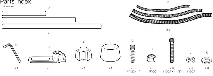
Before installation, locate the best possible attachment points for (D) foot bases, such as a seat bolt or any other existing screw, nut or bolt. If desired, you may drill your own attachment point using a bolt, washer and nut, or with a sheet metal screw.
